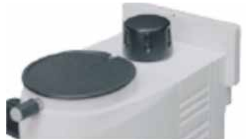
Photo above shows microscope light intensity control.
