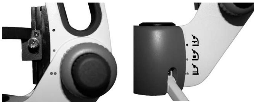
For proper stage ring adjustment, loosen the stage position thumbscrew to raise or lower the stage ring housing to line up with the desired stage position indicator marks. Tighten the thumbscrew to secure the stage assembly in place. The macro indicator marks are the *suggested* positions for viewing most macro specimens. The macro stage ring positions may have to be adjusted slightly to find the best working distance for unusual sized specimens.
